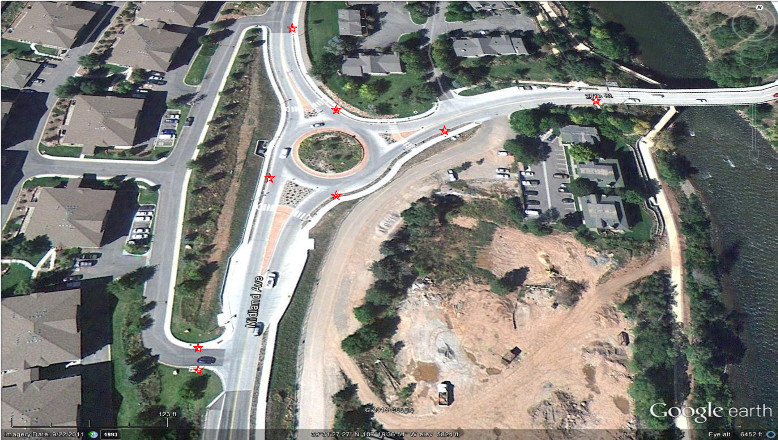
Figure 6. Existing Stormwater Conveyance Features. Locations indicated by a ★.
