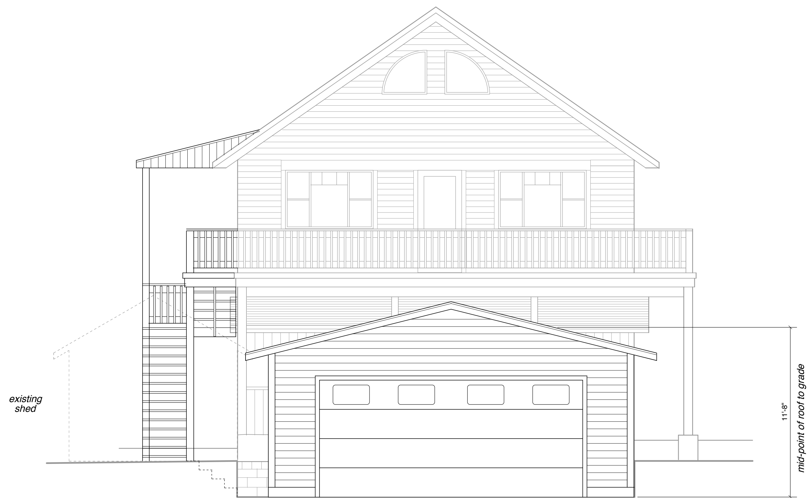
2 2-CAR GARAGE - WEST ELEVATION 1/4"=1'-0"
