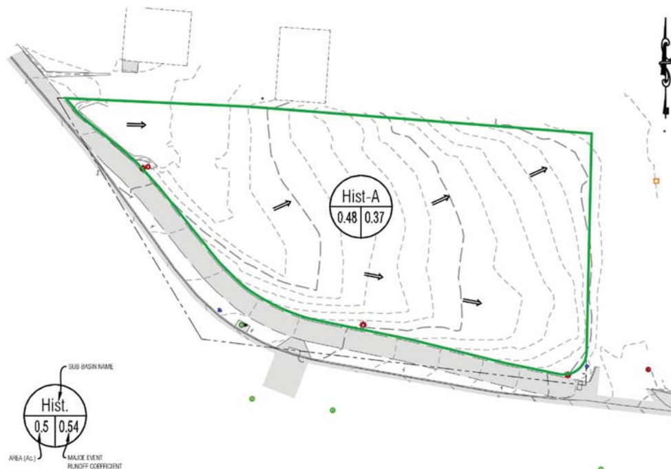
Figure 1: Historic/Existing Onsite Drainage Basins
