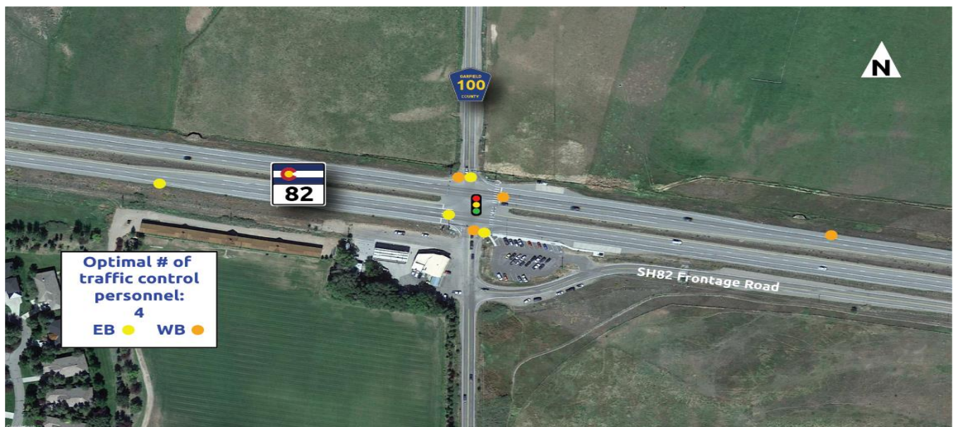
Figure 2.24 SH 82 Closure Point at CR 100
