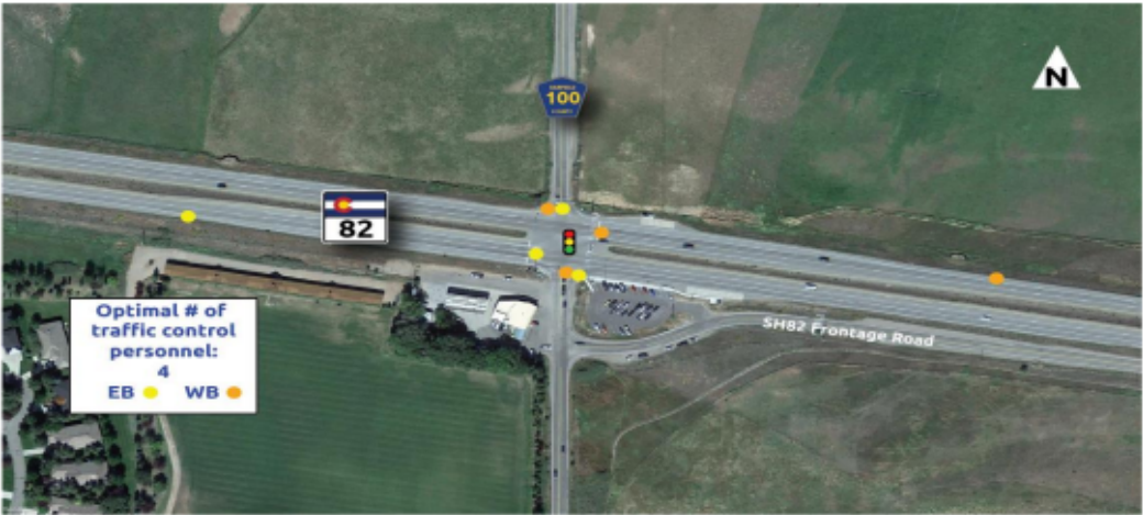
Figure 2.24 SH 82 Closure Point at CR 100
