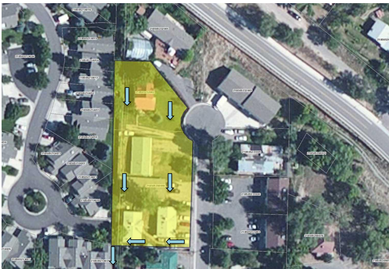
Figure 3: Existing Conditions & Runoff Patterns
