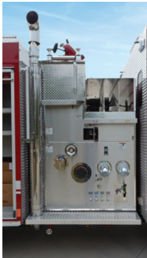
Shown with a traditional pump house configuration.
