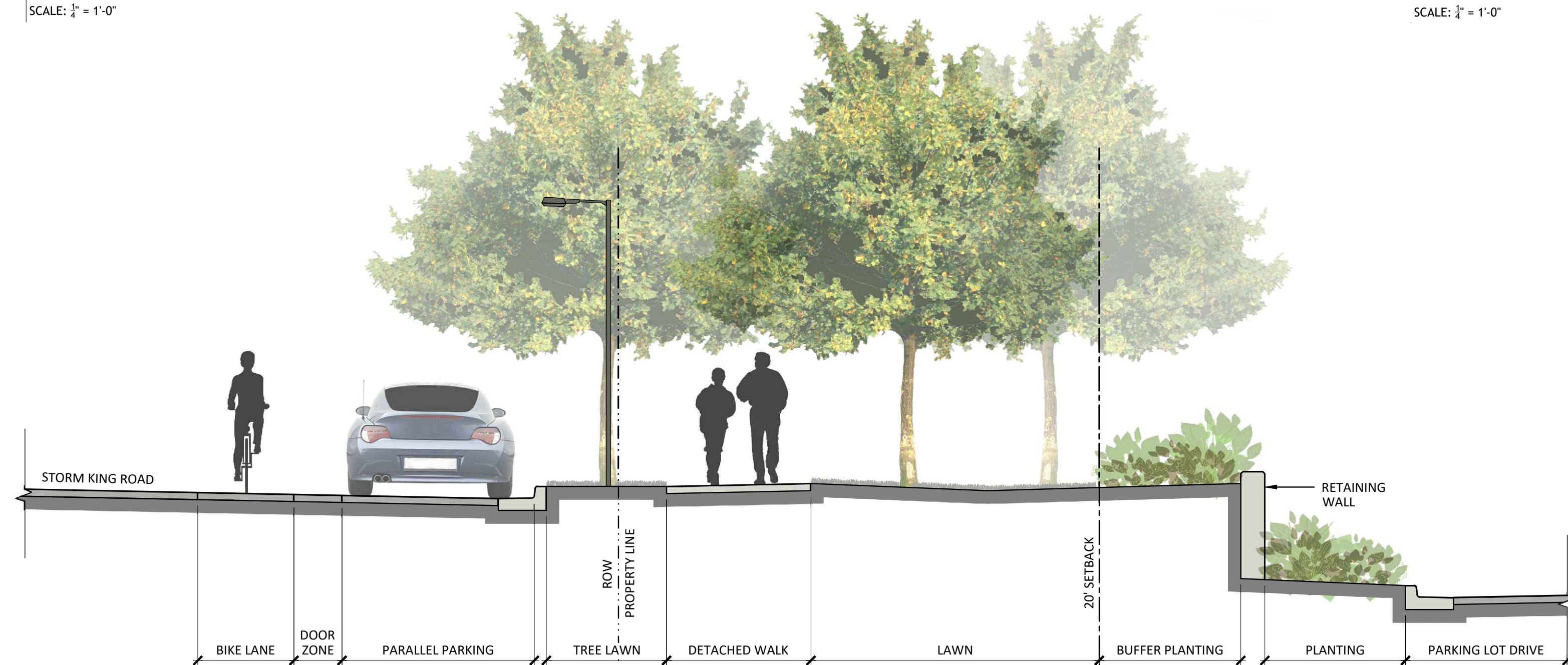
5 SECTION - STORM KING ROAD B SCALE: \frac{1}{2}'' = 1'-0''
