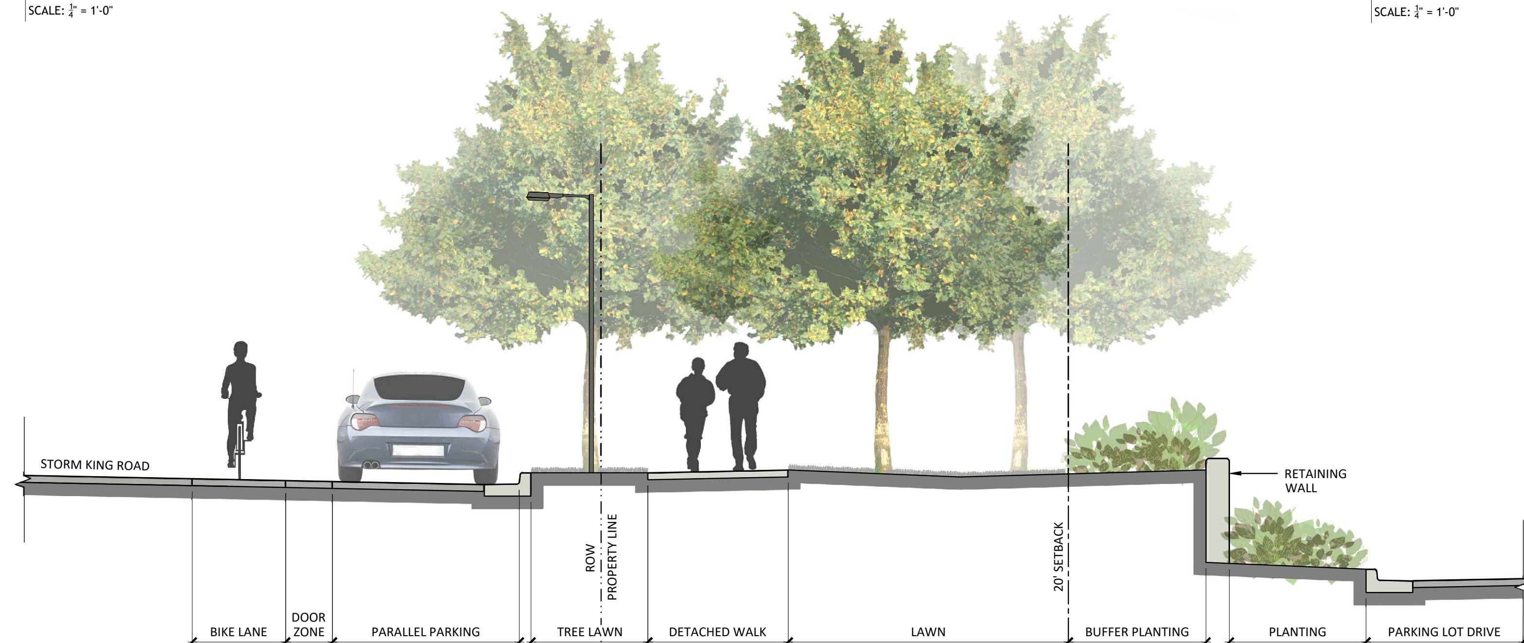
5 SECTION - STORM KING ROAD B SCALE: \frac{1}{4}'' = 1'-0''
