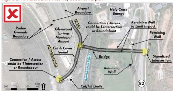
Figure 2-10 Alternative No. 16, South of Airport
