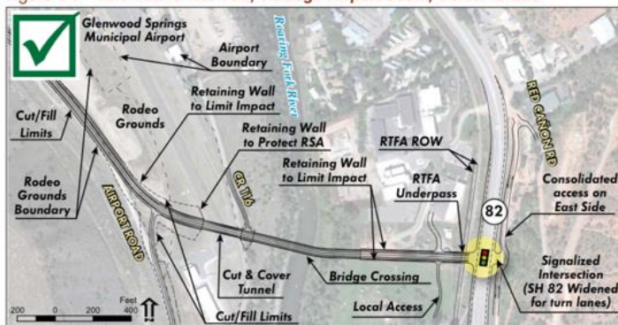
Figure 2-9 Alternative No. 10B, Through Airport South, Below-Grade
