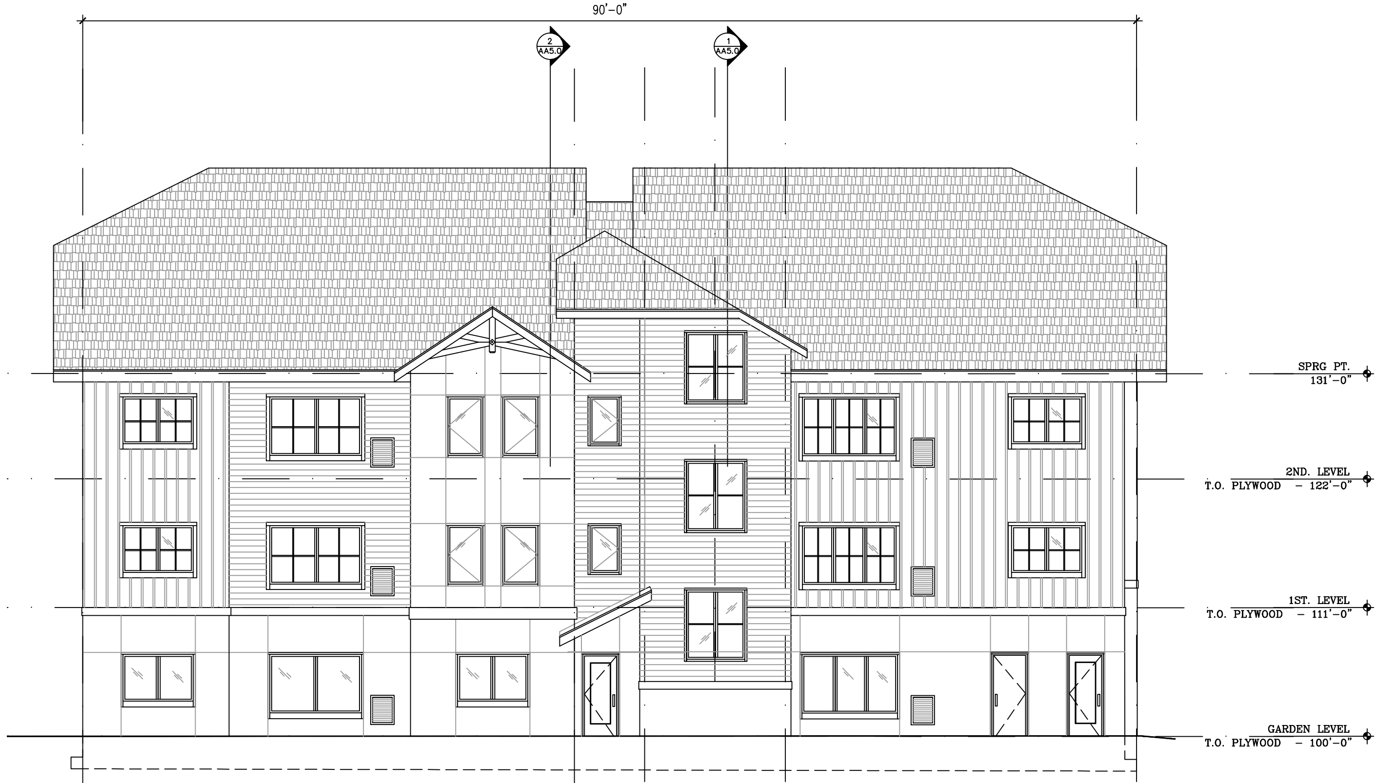
1 BUILDING A - WEST ELEVATION 1/8" = 1'-0"
