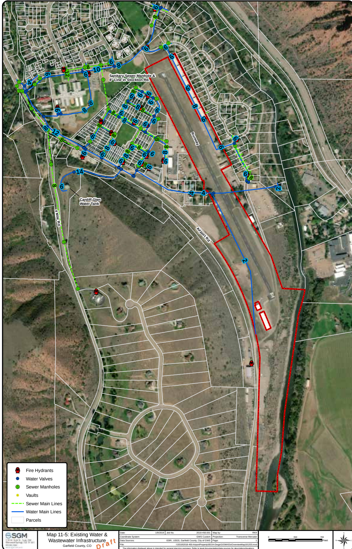
MAP II-4: EXISTING WATER AND WASTEWATER INFRASTRUCTURE
