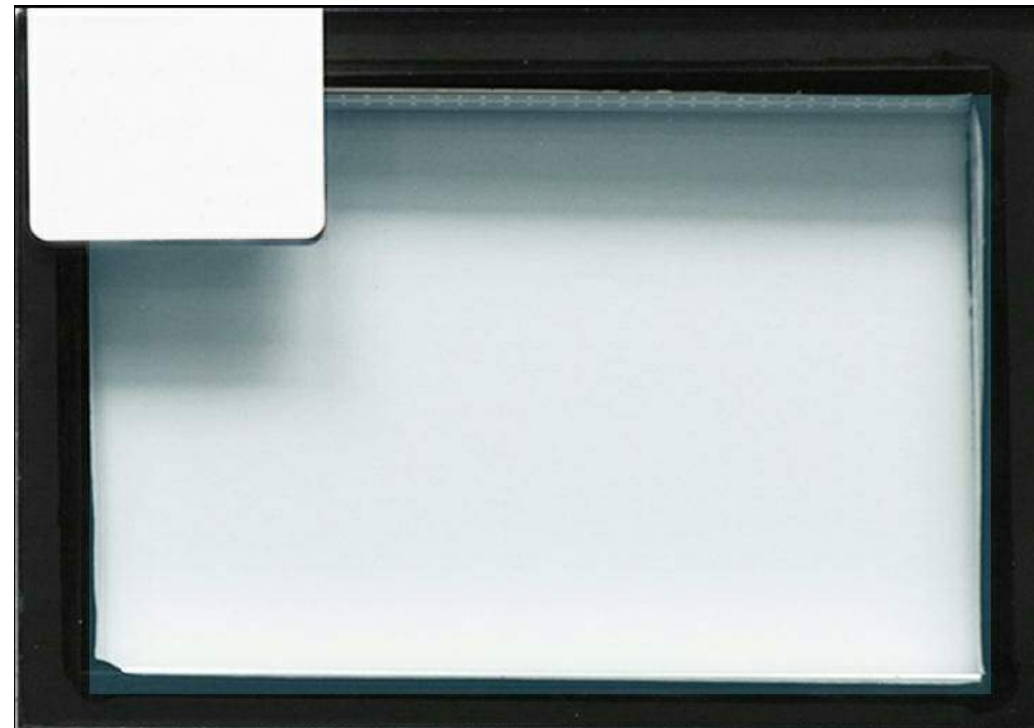
STOREFRONT VISION GLAZING - 1/4" SUNGUARD SNX 62/27 ON CLEAR, 1/2" AIR, 1/4" CLEAR
