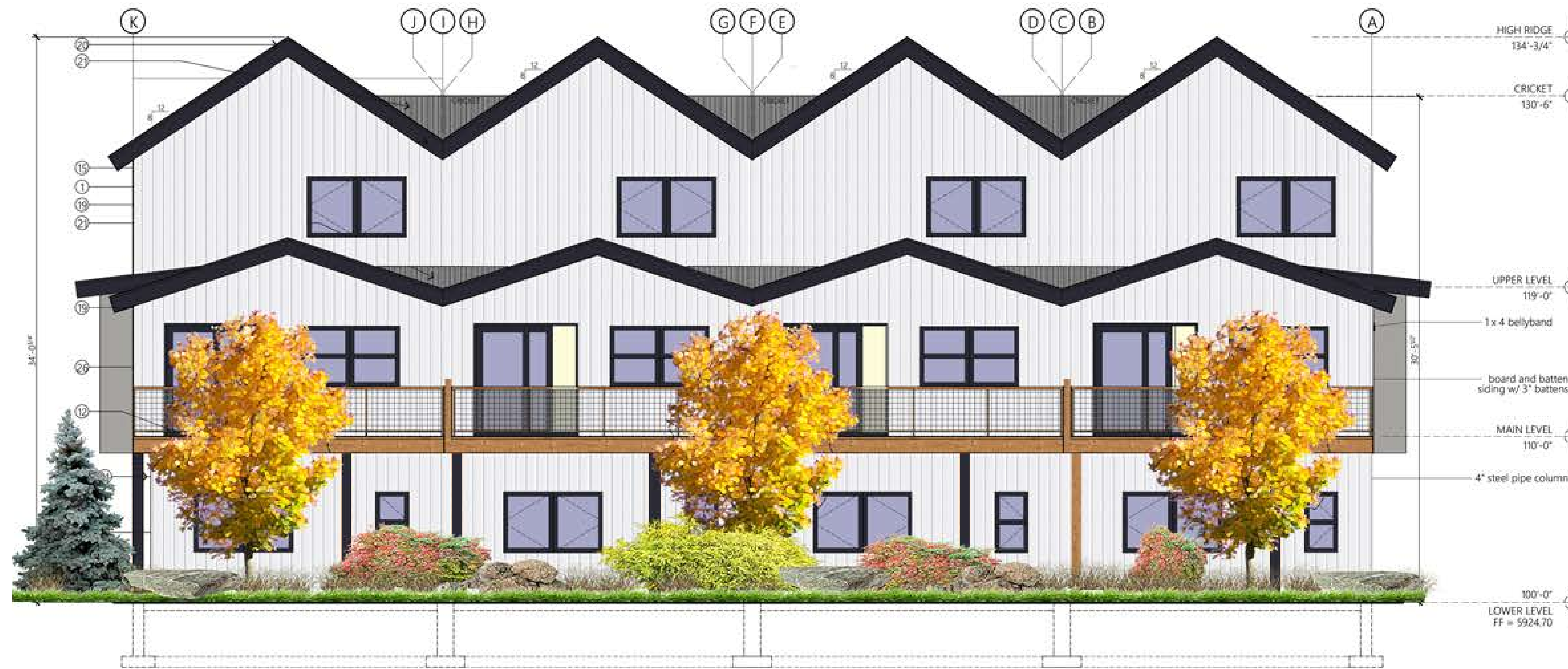
BUILDING '6' ELEVATION SCALE: 1/4" = 1'-0" NORTHWEST FACING
