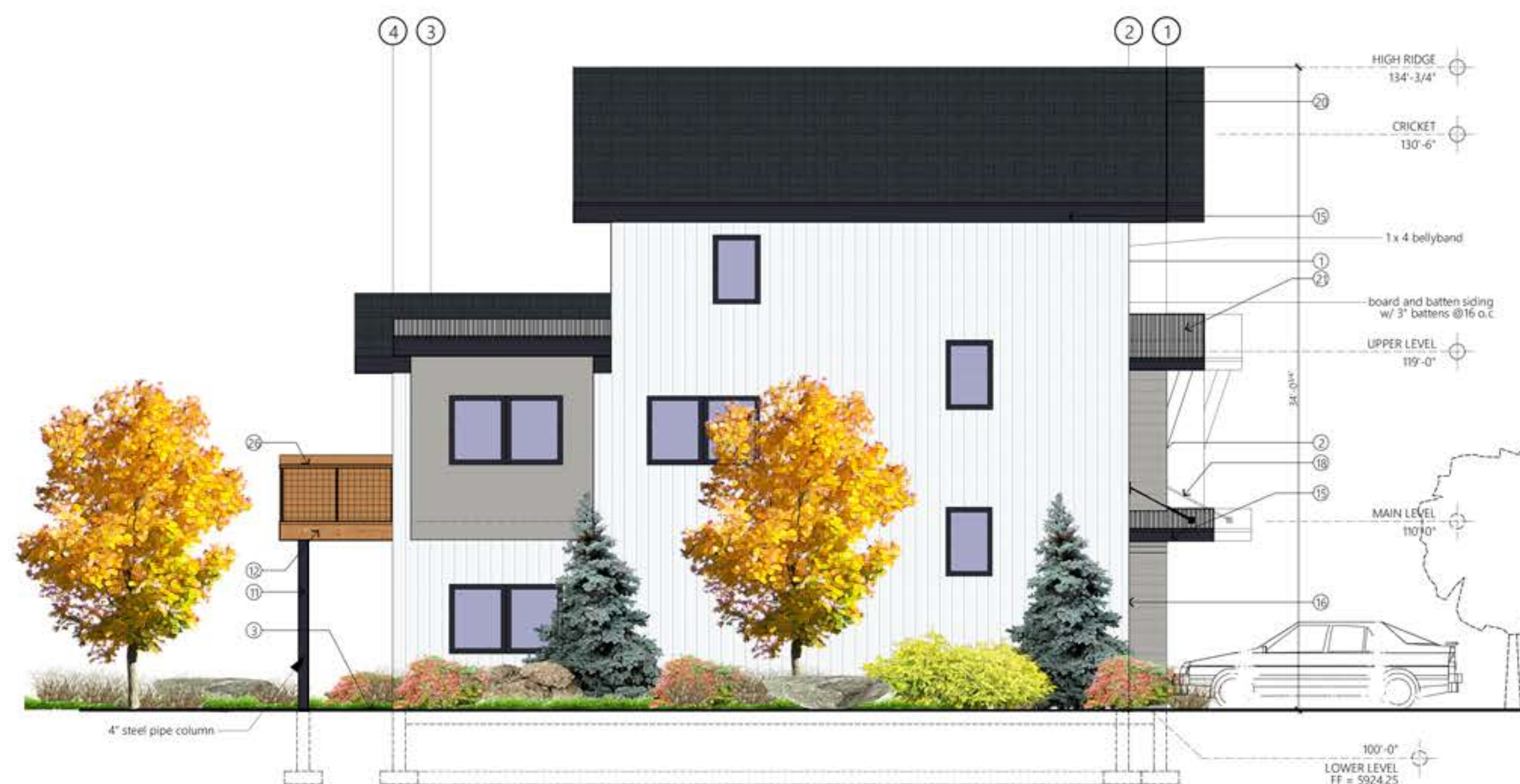
BUILDING '2' ELEVATION SCALE: 1/4" = 1'-0" NORTHWEST FACING END UNIT
