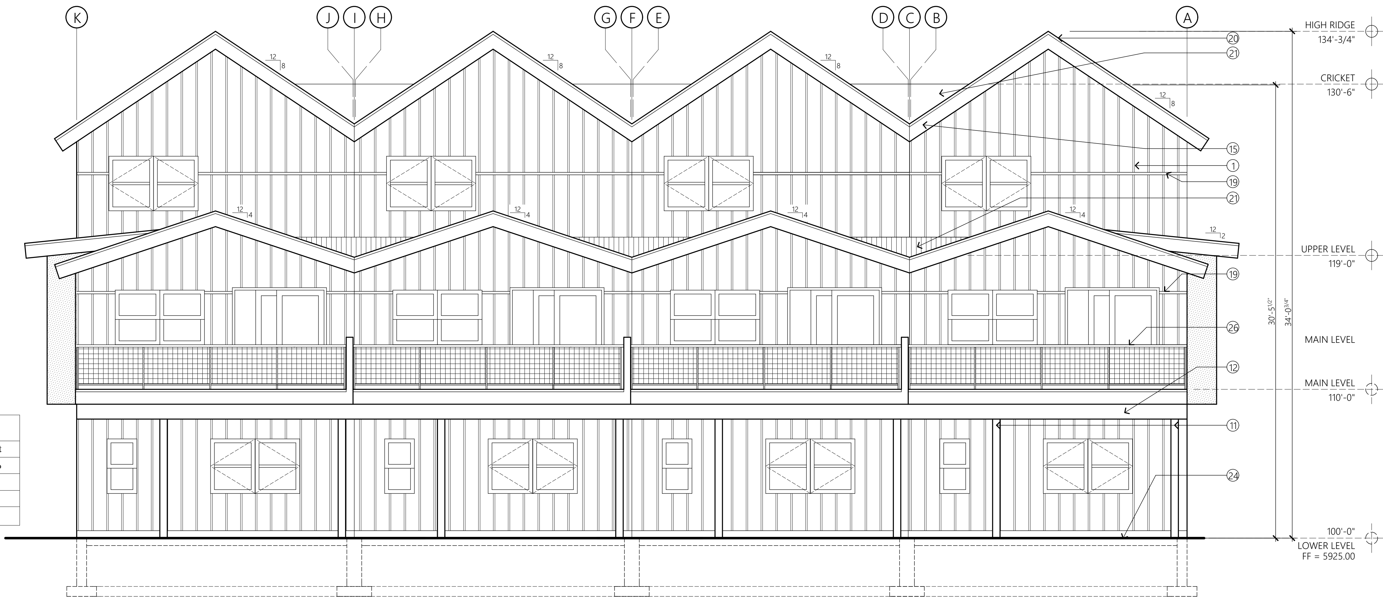
BUILDING '3' ELEVATION SCALE: 1/4" = 1'-0" SOUTHEAST FACING
