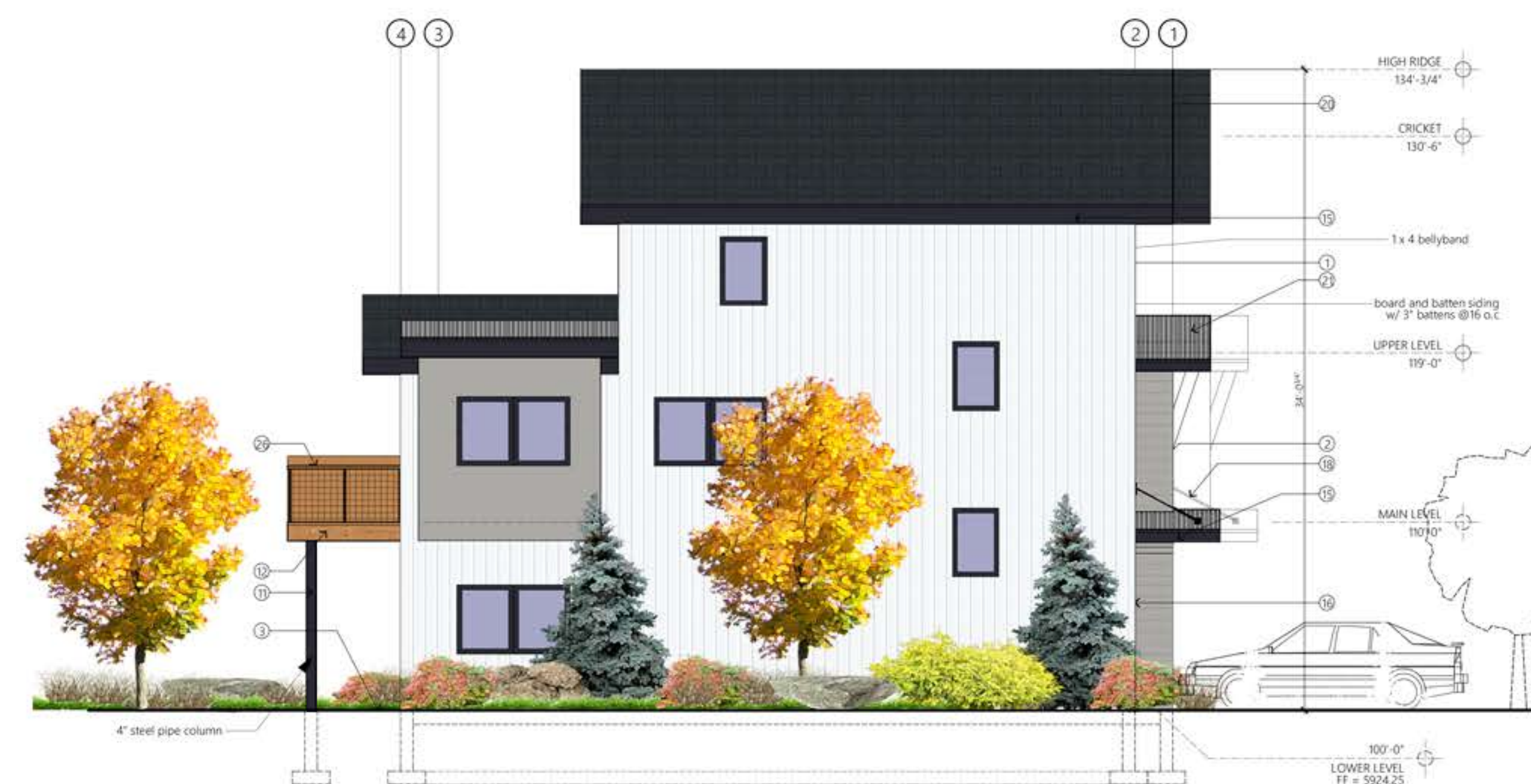
BUILDING '2' ELEVATION SCALE: 1/4" = 1'-0" NORTHWEST FACING END UNIT
