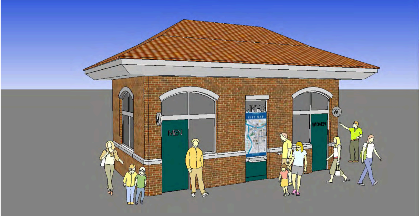
OPTION 2 - BRICK BASE WITH PRECAST CONCRETE BAND
