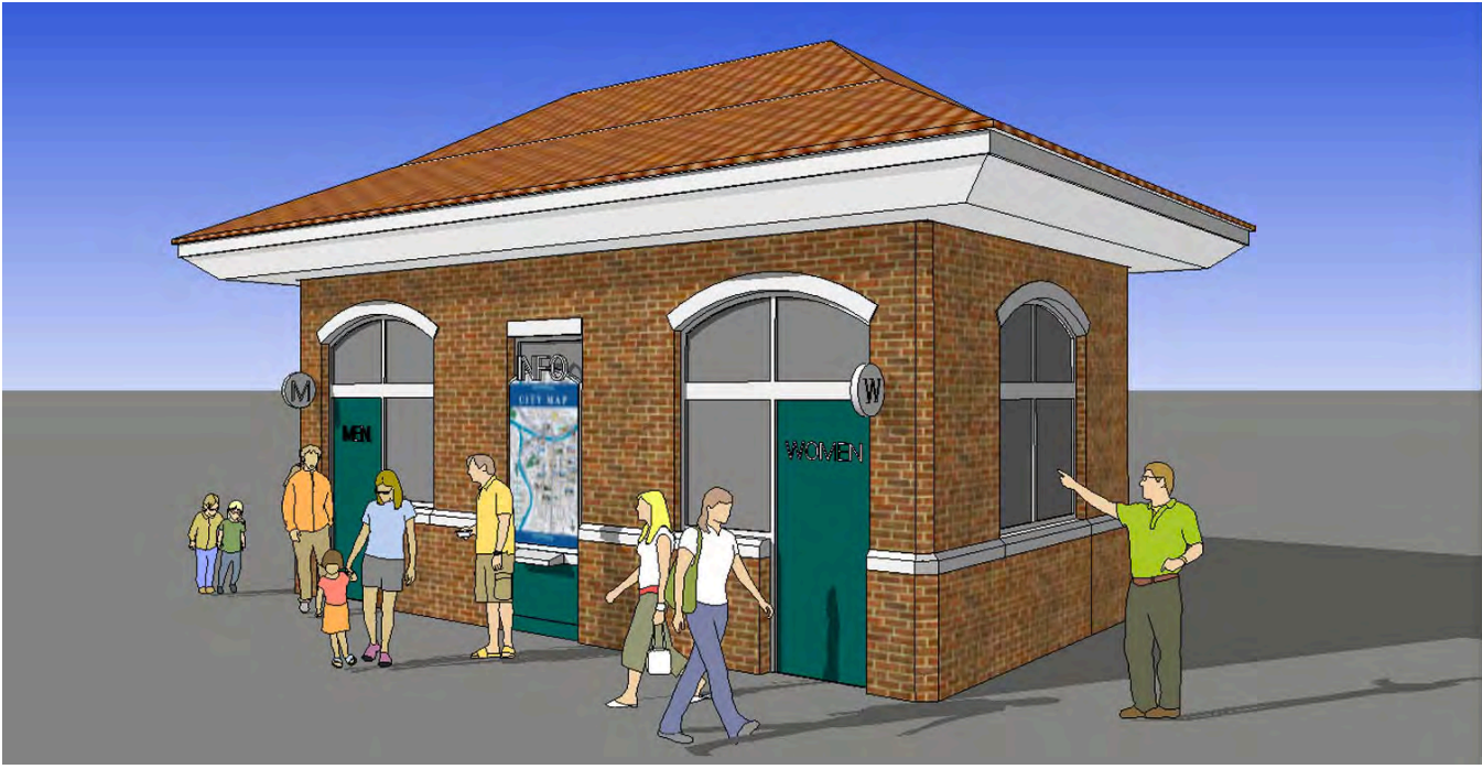
OPTION 2 - BRICK BASE WITH PRECAST CONCRETE BAND
